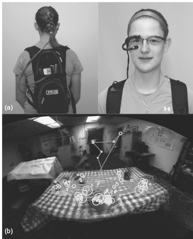
Figure 1 The RIT Wearable Eyetracker, Showing the Scene Camera and Eye Camera Mounted on a Lightweight Glasses Frame
