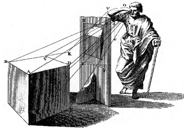
Figure 3 Basic Principle of Linear Perspective From Brooke Taylor, New Principles of Linear Perspective (1811)
