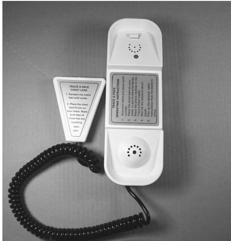
Figure 5.15 A transtelephonic ECG monitor provides a simple, effective solution for monitoring pacemaker patients from the comfort of their home. To transmit real-time ECGs, the patient simply dials the receiving center and places the telephone handset on the transmitter's cradle. These monitors typically use a center frequency of 1965 Hz with a deviation of 100 Hz/mV to convey a 0.5 to 100 Hz ECG signal detected through three chest electrodes that are dampened with water.
