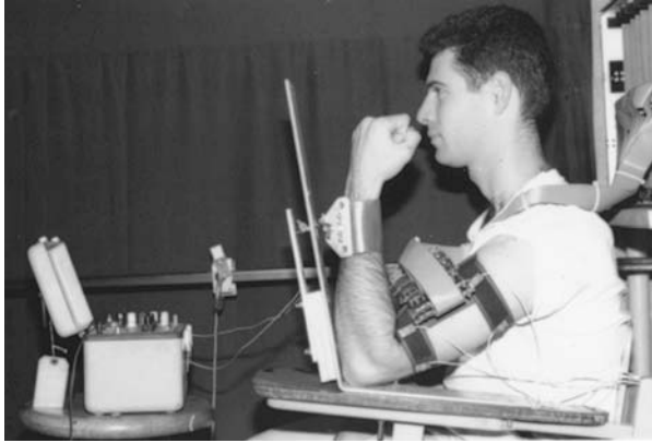
Figure 1.9 Eight high-input-impedance buffer arrays are used to detect muscle signals from 256 points for a high-resolution large-array surface electromyography system. Arrays of gold-plated pins soldered directly to array inputs are used as the electrodes.
