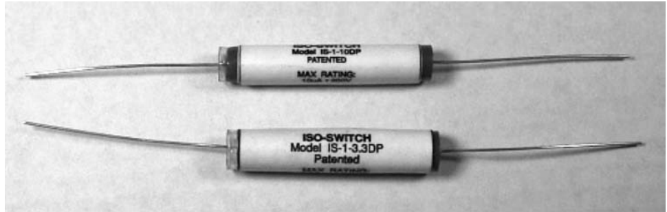
Figure 3.19 Ohmic Instruments' Iso-Switch patient-lead fault interruptors are two-lead semiconductor devices that can be placed, almost transparently, in series with every patient connection to break the patient circuit in case an overcurrent fault develops. Various models are available for different applications, with trip currents ranging from \pm 1 \mu\text{A} to \pm 100 \mu\text{A} . Various operating voltage ranges are also offered: \pm 325 \text{ V} for 115-V ac instruments, \pm 720 \text{ V} for 220-V ac equipment, and the DP (defibrillation-proof) series that withstands pulses of \pm 5 \text{ kV} for 10 ms.
