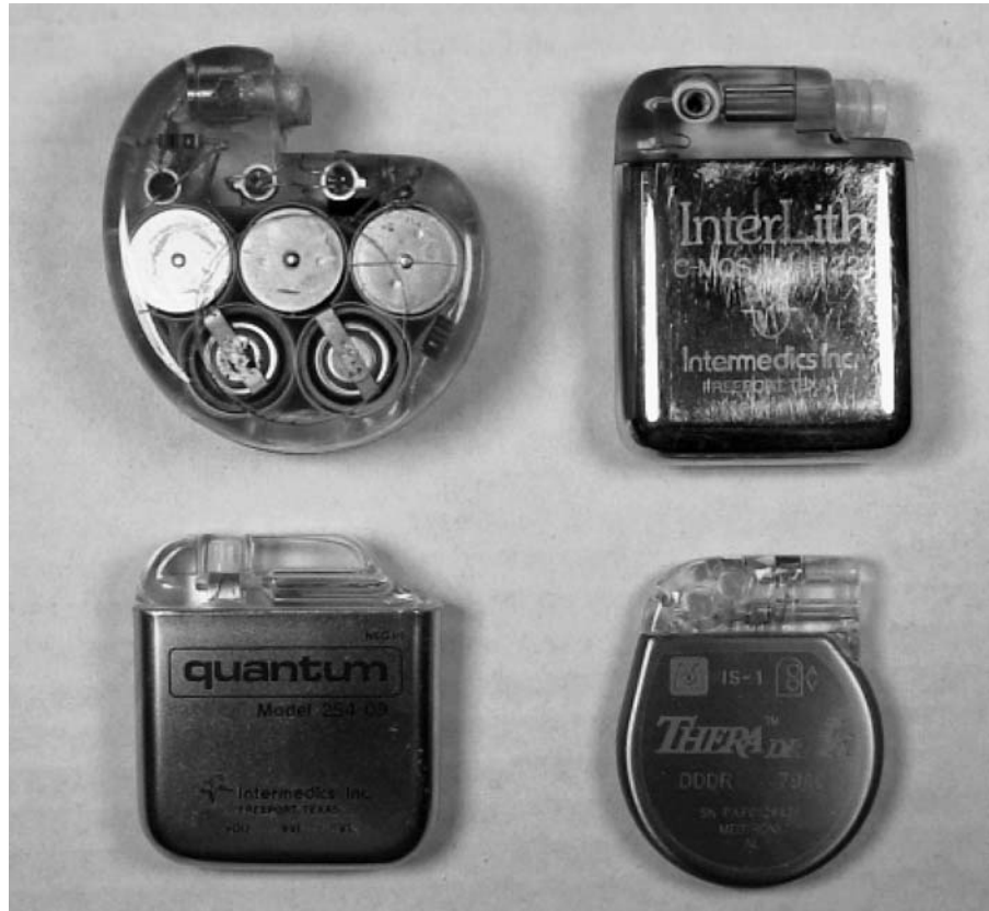
Figure 8.8 Evolution of implantable pacemakers. Top, left to right: Very early CCC VOO pacemaker powered by six mercury cells, Intermedics InterLith VVI with CMOS circuitry and powered by a lithium cell. Bottom: Intermedics “Quantum” programmable VVI/VVT pacemaker, a modern Medtronic Thera DDDR pacemaker.
