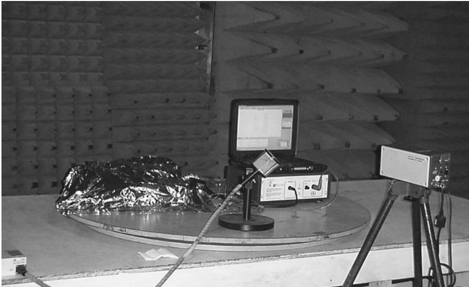
Figure 4.22 A prototype implantable-device programmer is being tested to assess its susceptibility to radiated EMI. An implantable device and a simulator need to interact with the device under test to assess its behavior. These test accessories are placed under the aluminum foil shield. A TV camera relays the image from the programmer's computer screen to the control station outside the shielded room.
