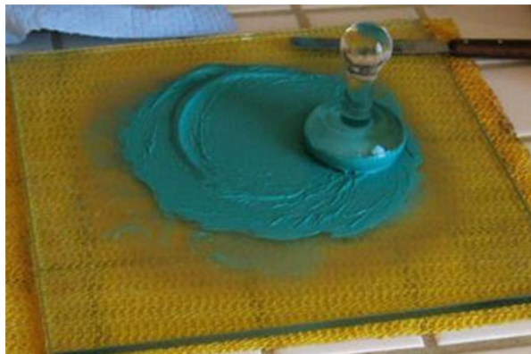
Fig. 4.9 Schematic representation of solid sample preparation mulling technique
