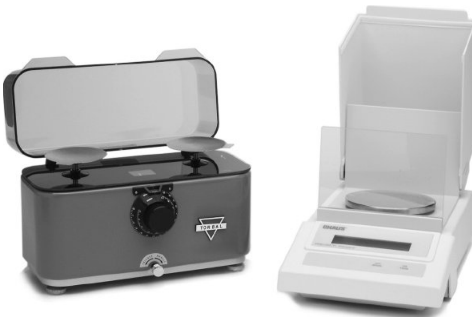
FIGURE 3.3 • Torbal torsion balance and Ohaus electronic balance. (Courtesy of Torbal and Ohaus.)
