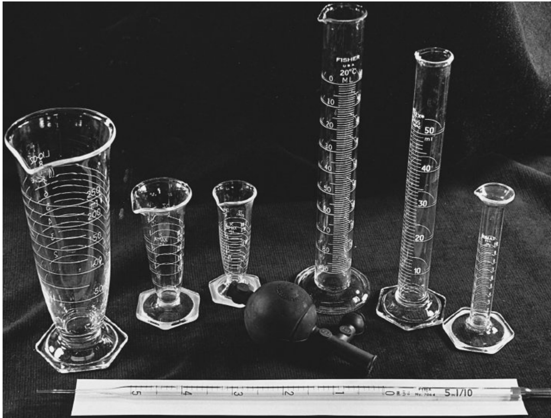
FIGURE 3.1 • Examples of conical and cylindric graduates, a pipette, and a pipette-filling bulb for volumetric measurement.
