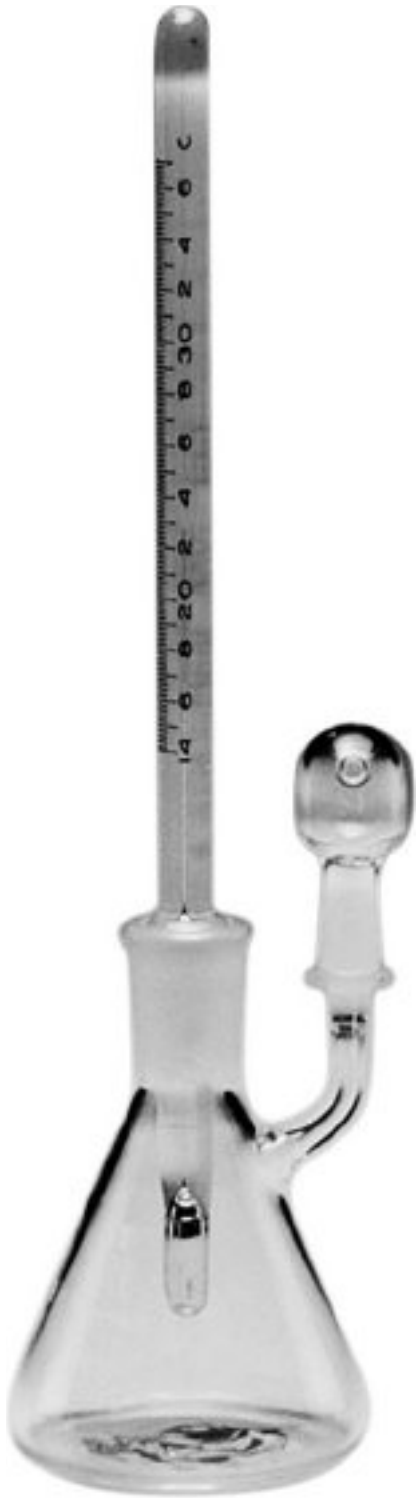
fiGURe 5.2 • Example of a pycnometer affixed with a thermometer. Pycnometers are used to determine the specific gravities of liquids at specific temperatures. See text for additional discussion. (Courtesy of Kimble/Kontes Glass.)
