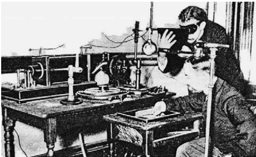
FIGURE 21.2 A Pioneer Radiologist Testing His Fluoroscope by Examining His Own Hand, Fully Exposing Himself and His Patient in the Process
