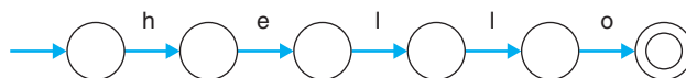
■ FIGURE 5.2 The beginning of a finite automaton to look for the substring “hello”
