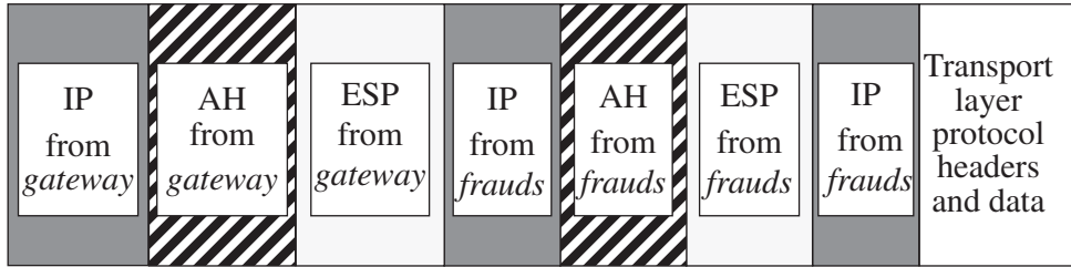
Figure 10–5 An IPsec-protected packet going through nested tunnels. The filled rectangles represent headers. The rightmost IP header and the following data constitute the original packet. The IPsec mechanisms add the ESP, AH, and IP headers of frauds and forward the packet to gateway . This is the first SA and is in tunnel mode. The host gateway adds the ESP, AH, and IP headers shown, putting the packet into the second tunnel mode SA.
