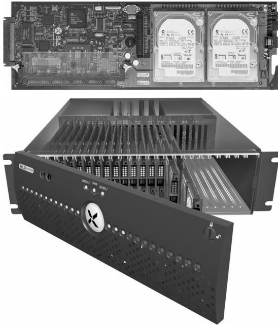
Blade and Rack of Beowulf Cluster
